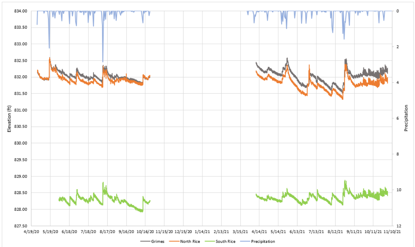
Figure 3-7 2020 and 2021 Pond Water Levels
